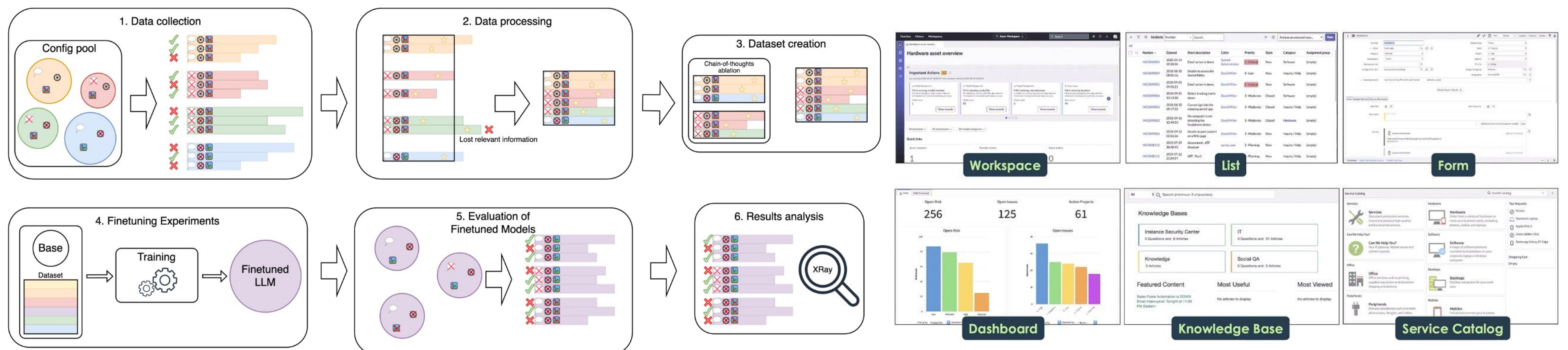
Figure 2. Our generic pipeline: 1) Trajectories are generated using different configurations (Chain-of-thoughts: 🧠, use error logs: 🗑️, use screenshot: 📸) and different LLMs (highlighted by different colors). 2) Only the successful trajectories are kept. As each prompt is truncated to fit in our trained model's window, some key information (🗑️) might get lost in the process. Those samples are discarded. 3) The pipeline now has a pool of data, which can be used to build training sets with different properties. Here, we build an ablation dataset that separates data with and without chain-of-thoughts, and a dataset that merges both. 4) After selecting a dataset, we train our model starting from a base model to make a stronger finetuned LLM. 5) The latter is used along with different agent configurations to assess the finetuning quality. 6) Finally, we can leverage AgentLab's tools to manually analyze the traces produced by the model.
